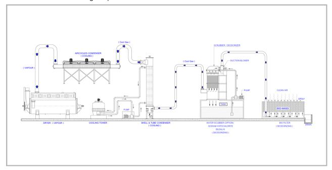
The hot vapor exhaust from the drier is quite smelly and must be treated by condensing (cooling) to water.
