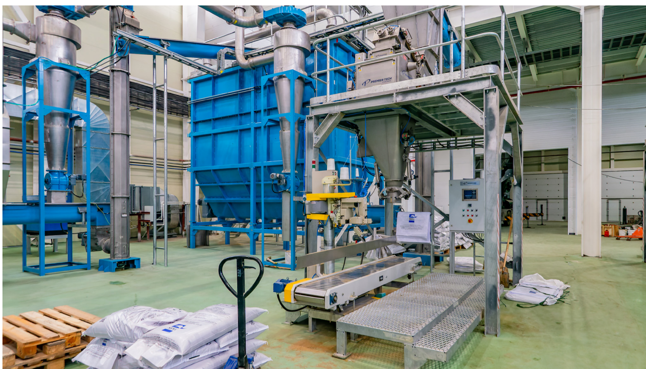
OFP 504 installed at PCF Yuzhno-Kyriiski Rybocombinat Co., Ltd., Russia 2018. Capacity: 504 tons raw material input/24 hrs
