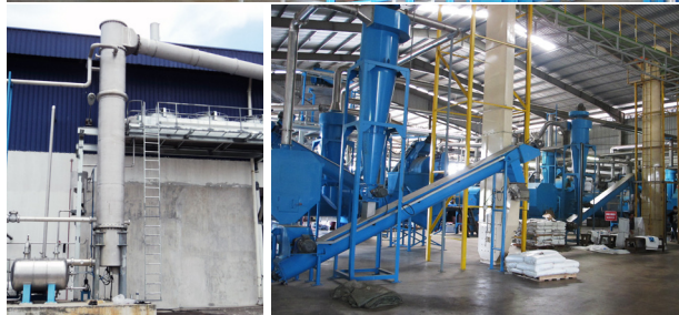
3 x LFP 160 installed at QL Endau Marine Products, Johor, Malaysia 2011 Capacity: 160-180 tons raw material input/24 hrs
