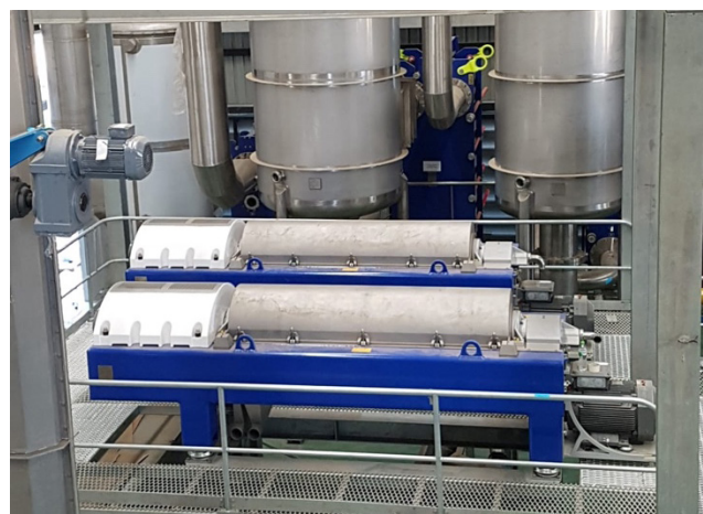
Three phase decanter type Alfa Laval, to separate sludge, oil and stick water from the press water.
