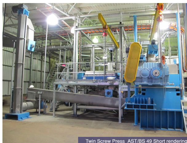
Twin Screw Press AST/BS 49 Short rendering (Installed at Scone, Australia for Primo Quality Meats.)
