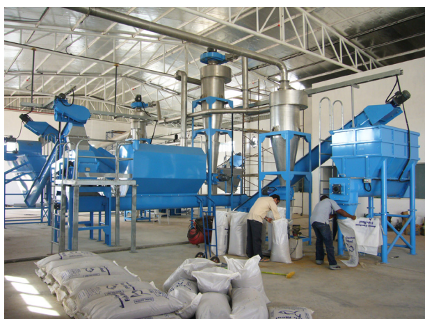
LFP 24 installed at Bahr Al-Arab Factory in Umm Al-Quwain, UAE 2012 Capacity: 24-30 tons raw material input/24 hrs
