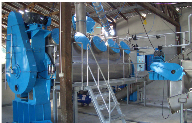
Rotary disc dryer type AST/TST 4.4 SS/V/FG raw material input 24 tons per 24 hrs (Thailand)
