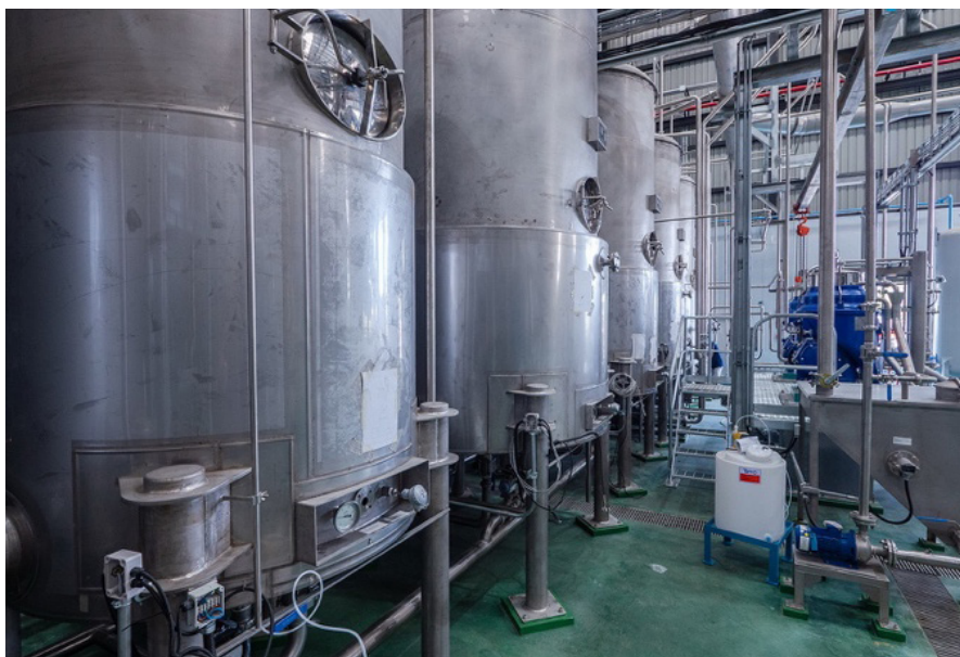
Separator purifier with stainless steel oil processing tanks.
