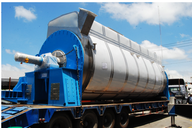
Very good finish, painting and stainless cladding for insulation.
