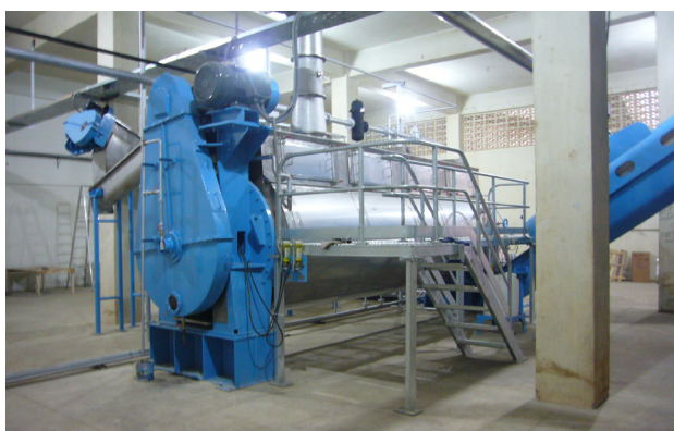
Rotary disc dryer type AST/TST 10.0C raw material input 55 tons per 24 hrs (Pakistan)
