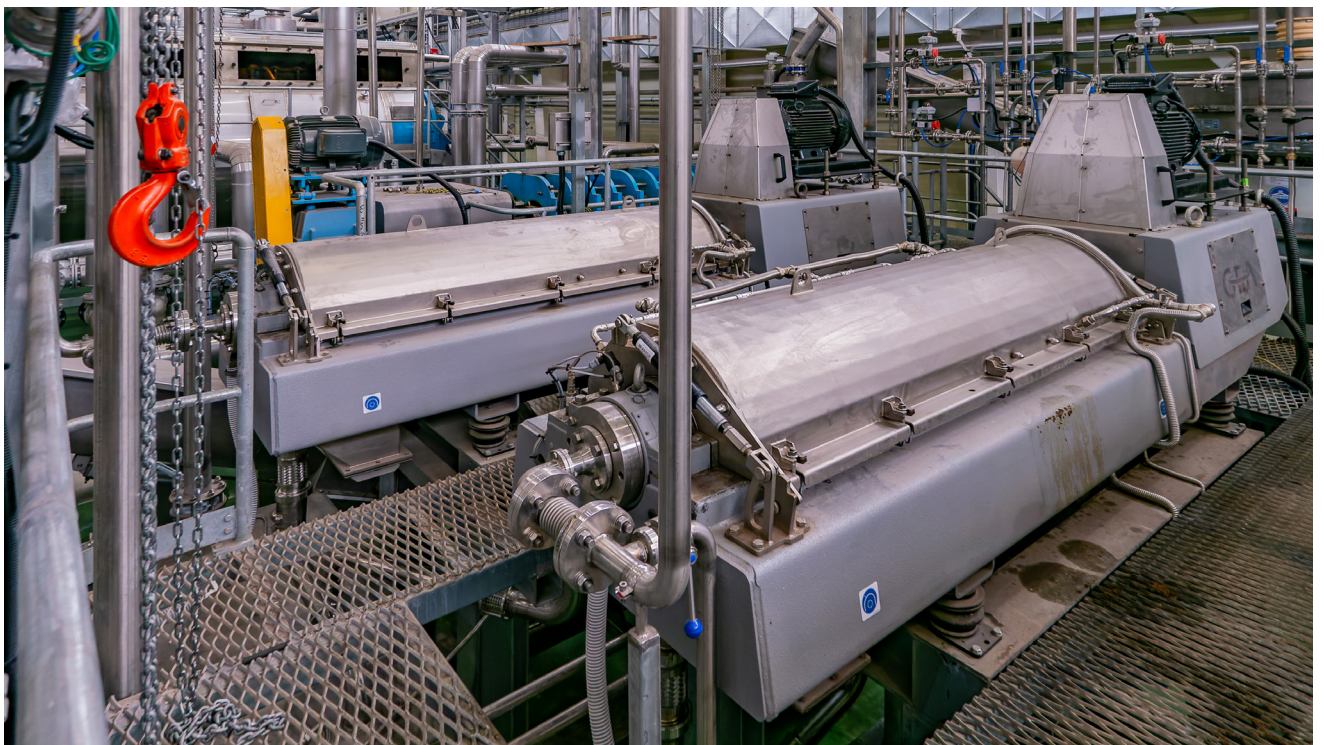
OFP 504 installed at PCF Yuzhno-Kyriilskiy Ryibocombinat Co., Ltd., Russia 2018. Capacity: 504 tons raw material input/24 hrs
