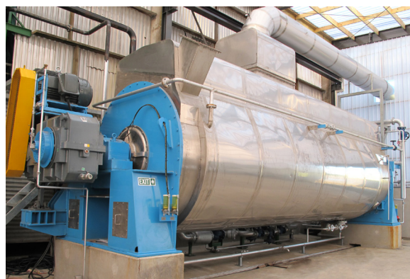
Rotary disc dryer type AST/TST 40.0 raw material input 220 tons per 24 hrs (New Zealand)
