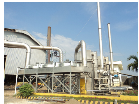
Air cooled condenser and Water scrubber-deodorizer.
