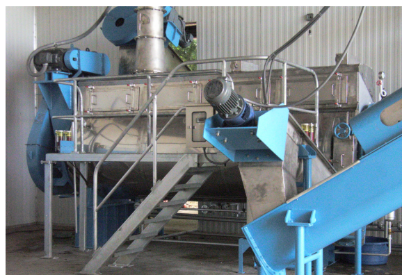
Rotary disc dryer type AST/TST 4.4 raw material input 24 tons per 24 hrs (Nicaragua)
