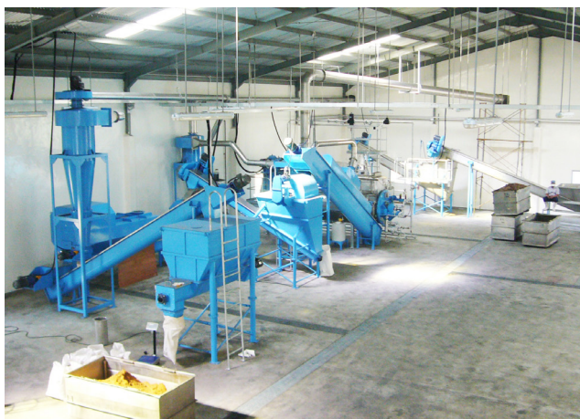
LFP 24 installed at PT. Aneka Tuna Indo in Pasuruan, Indonesia 2011 Capacity: 24-30 tons raw material input/24 hrs
