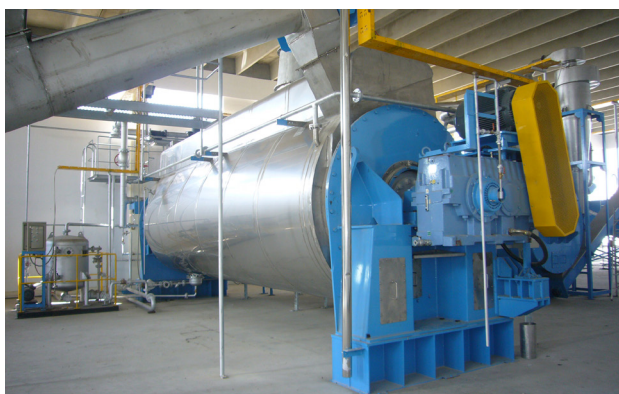
Rotary disc dryer type AST/TST 30.0 raw material input 160 tons per 24 hrs (Pakistan)
