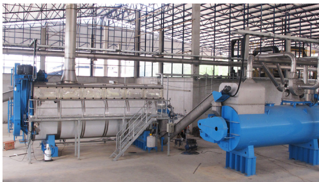
LFP 55 installed at Qaswa Feed & Allied Products, Karachi, Pakistan 2014 Capacity: 55-60 tons raw material input/24
