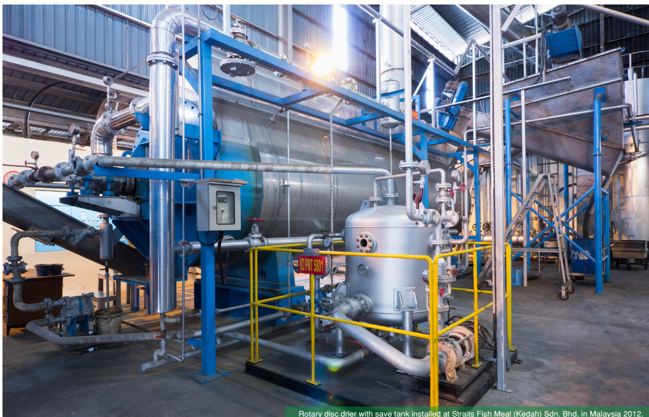
Rotary disc drier with save tank installed at Straits Fish Meal (Kedah) Sdn. Bhd. in Malaysia 2012.
