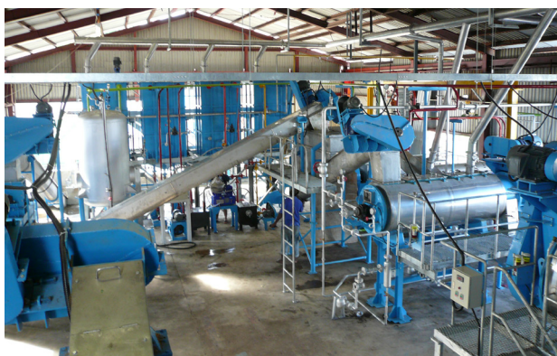
OFP 55 installed at Soltuna Limited, Honiara, Solomon 2007 Capacity: 55-60 tons raw material input/24 hrs
