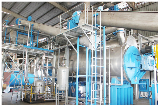
LFP 90 (plant no.2) installed at Thanh Hoa Agricultural JSC, Vietnam 2013 Capacity: 90-100 tons raw material input/24 hrs
