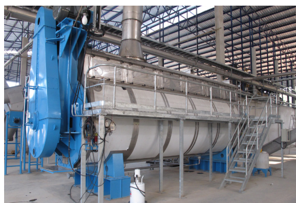
Rotary disc dryer type AST/TST 24.0 raw material input 120 tons per 24 hrs (Thailand)
