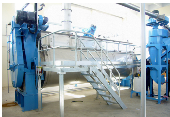
Rotary disc dryer type AST/TST 10.0C raw material input 55 tons per 24 hrs (Indonesia)
