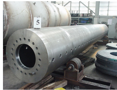
Special high grade rotor pipe from Europe made in one piece.
