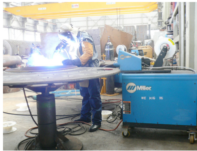
Welding with MIG flux core /CO2 the best method for quality welding.
