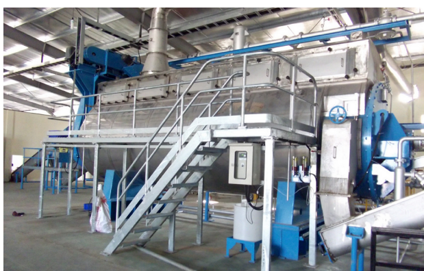
Rotary disc dryer type AST/TST 16.0 raw material input 90 tons per 24 hrs (Vietnam)
