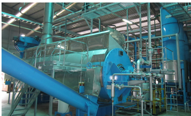
OFP 120 installed at Travel Investment and Seafood Corporation (TRISECO), An Giang, Vietnam 2011. Capacity: 120-140 tons raw material input/24 hrs.
