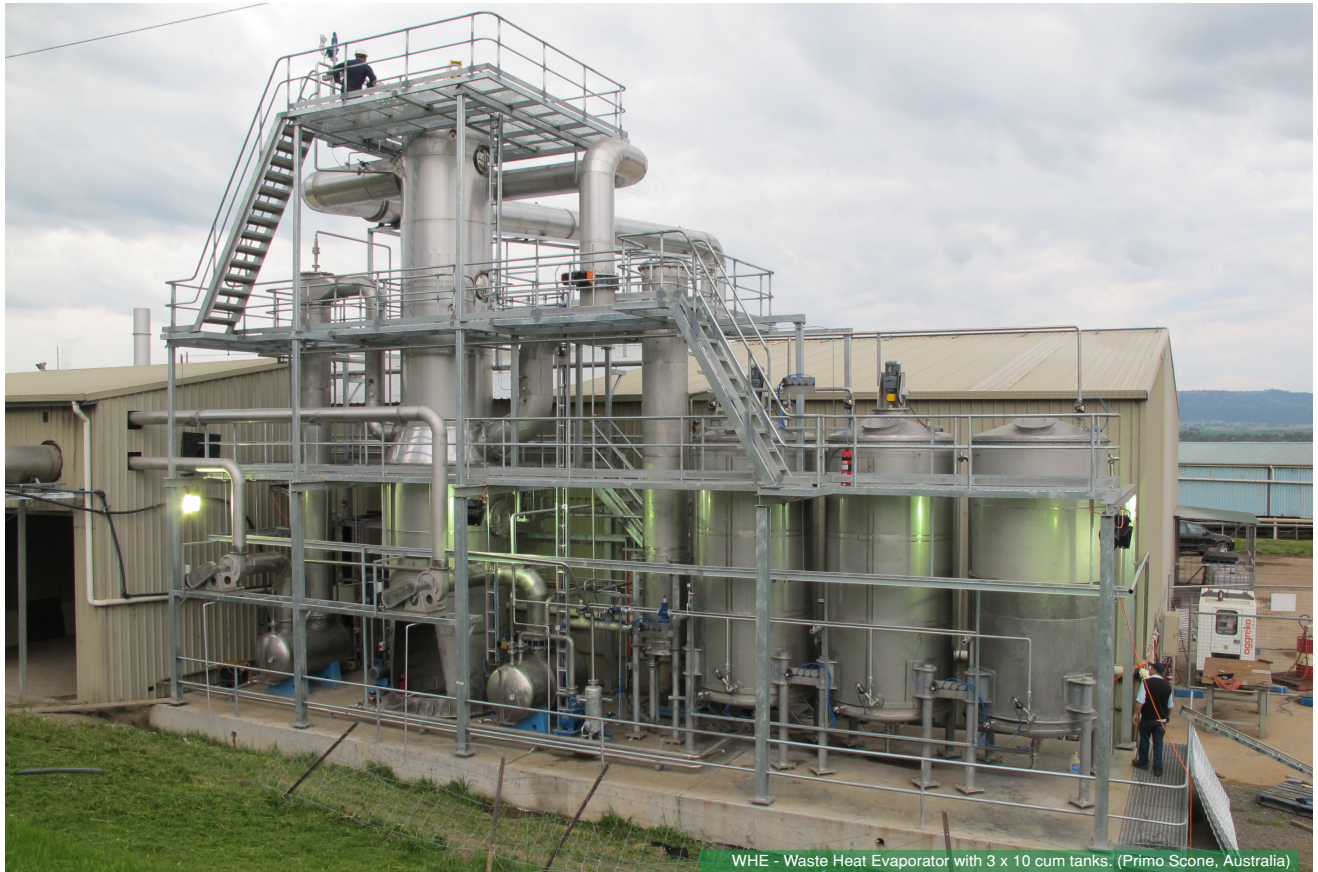
WHE - Waste Heat Evaporator with 3 x 10 cum tanks. (Primo Scone, Australia)
