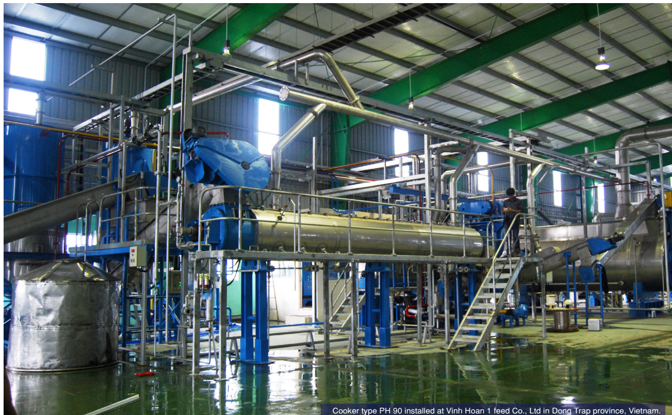
Cooker type PH 90 installed at Vinh Hoan 1 feed Co., Ltd in Dong Trap province, Vietnam.
